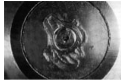
Example of a damaged SLC
