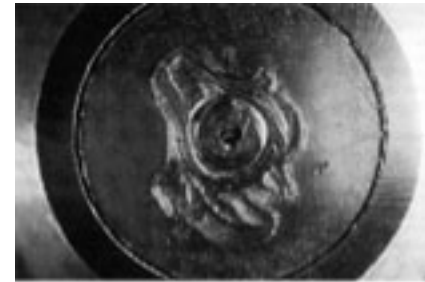
Example of a damaged SLC
